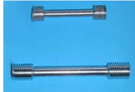
Probetas ASTM E8M:
