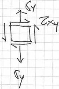
$$\sigma_y = \sigma_M + \sigma_H = 122.16 \text{ MPa} \quad (t = 2.5 \text{ mm})$$
