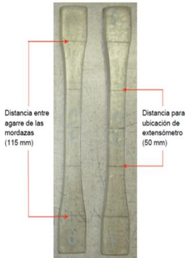
Probeta resina (ASTM D638)
